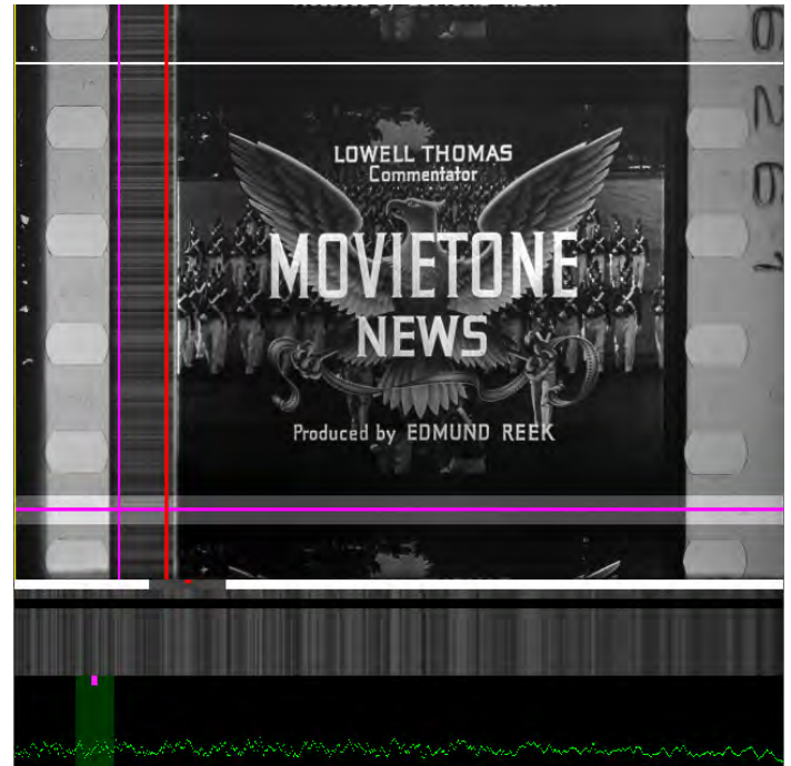
DIGITIZING OPTICAL SOUND. A variable density optical sound track is outlined by bounding boxes to the left of the 35mm film image.
